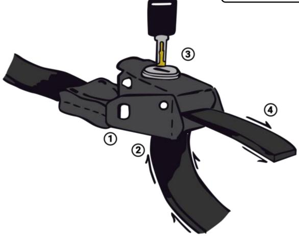
1. Push button and lift lever to open lock.
